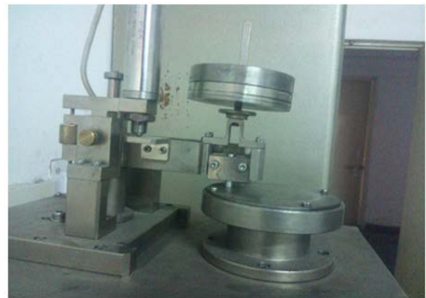
Fig. 2: Dry sliding wear machine used in present work.
